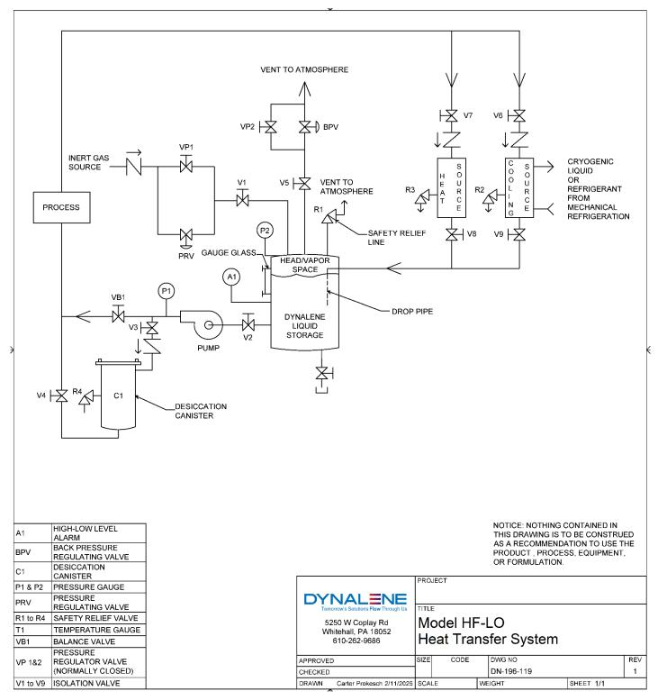
Figure 1. Basic Dynalene HF-LO heat transfer system.
