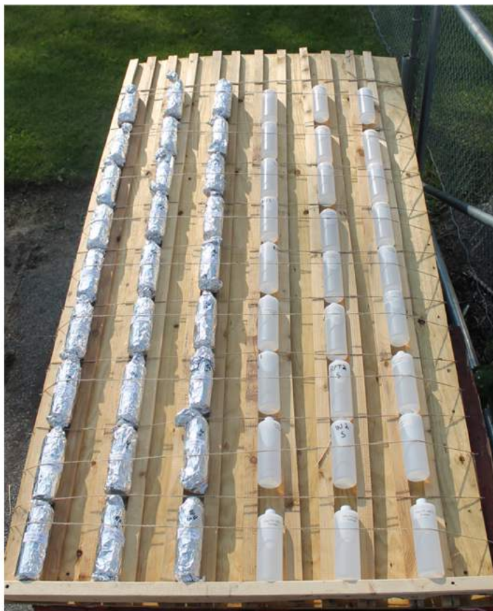
Figure 3: Fully exposed and foil-protected HDPE bottles on plywood rack.
