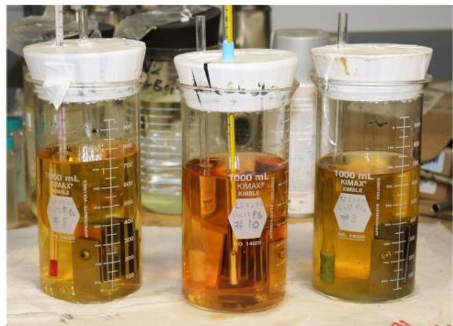
Figure 1: ASTM D1384 glassware with coupons in glycol-water mixture.
