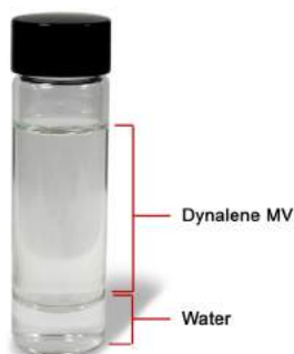
Figure 1: Dynalene MV-water two-component system in equilibrium at T = 23^{\circ}\text{C} .
