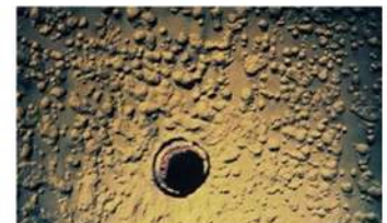
Figure 10: Cavitation causes bubbles and gas pockets on the surface [13]
