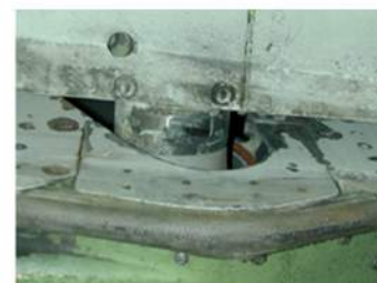
Figure 14: Fretting corrosion at highly loaded surfaces [14]
