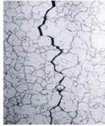
Figure 11: Intergranular SCC in Inconel heat exchanger tube [13]
