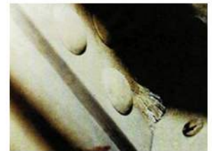
Figure 6: Exfoliation in Al alloy based aircraft component [13]
