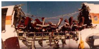
Figure 12: Corrosion Fatigue leading to failure of aircraft [14]
