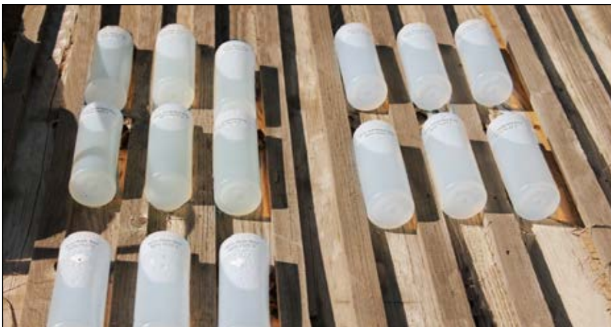
Figure 2: 50% glycol solutions with > 11 weeks of exposure. PG samples are the top six bottles on the left side.
